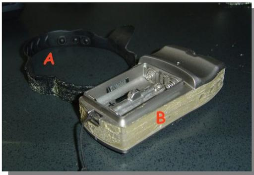
**FIRST REMOVE THE BATTERIES!** Carefully remove the “Rubber band” (A) from around the case. The adhesive is gummy and messy so take care. I used a knife blade to carefully lift and remove the band ... taking care not to cut the band during the process. There will then be a residue of the adhesive covering a clear vinyl tape around the joint (B).
