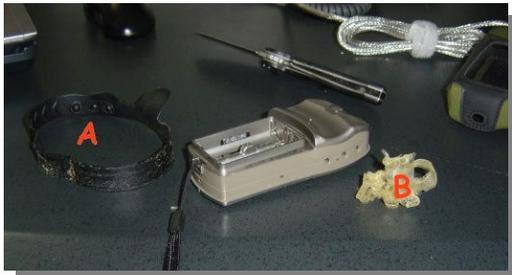
Next carefully remove the gummy adhesive and the clear vinyl tape from around the seam. This will leave you with a pile of “gunk” (B). Care should be used not to get this mess everywhere ... this would be a good time to use something to clean your hands to keep from smearing this everywhere.
